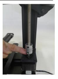
Let the lead screw snap into the coupling and the motor shaft is also aligned with the lead screw. Tighten the top wire
