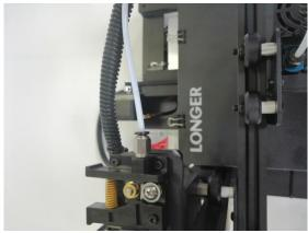
3. Because the end of the consumables in the nozzle will be deformed by heat, if the end deformed consumables are directly pulled out, it may be stuck to the pneumatic joint or the limit switch for damage detection. (The limit switch for the broken material detection is single. Towards).
