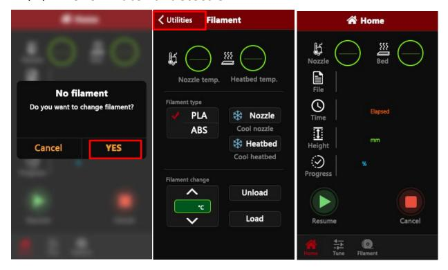
At this point, pull the Teflon tube out of the extruder end, take out the material, refill the consumables to the nozzle, click YES, after replacing the material, click Utilities, and finally click Print to start, the model will print.
