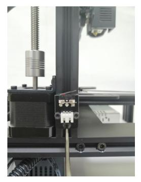
Z-axis limit opening installation is about 12mm from the base (this is adjustable)
