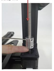
Adjust the screw movement by adjusting these two screws. The two screws cannot be tightened too tightly. Turn the coupling by hand to adjust the movement of the lead screw.
