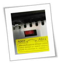
If the access voltage is 220V, please adjust the power supply in the control box to 220V, please be sure to confirm before powering on. Otherwise it will burn the power
