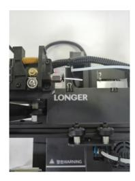
2. When withdrawing the consumables, before the end of the consumables reaches the pneumatic joint, we will usually pull the Teflon directly from the Teflon and cut the end of the consumables.
